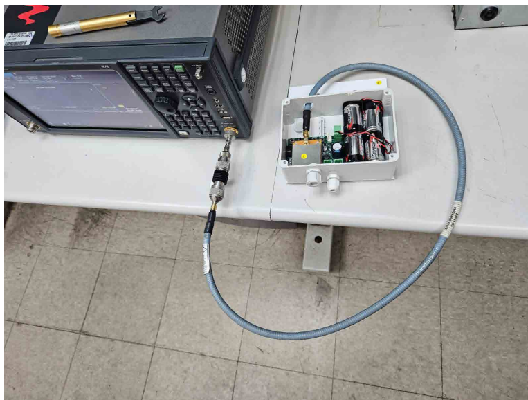
Picture 3 Conducted spurious emission test setup.
