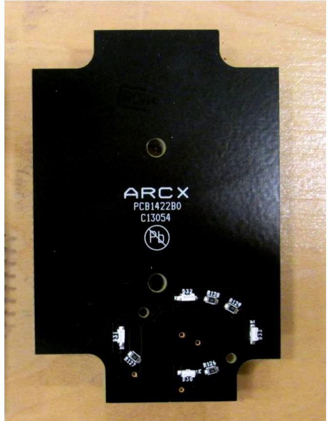
Board #3(RFID card reader antenna) as seen in photos EUT – Internal view 3-4 Side 2
