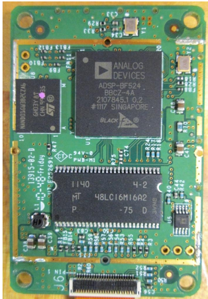
Board #1 (fingerprint reader board) as seen in photos EUT – Internal view 1-4, Side 2, shield off.
