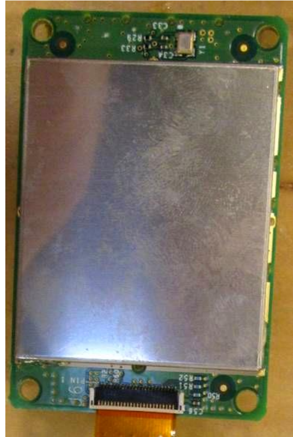
Board #1 (fingerprint reader board) as seen in photos EUT – Internal view 1-4 Side 2
