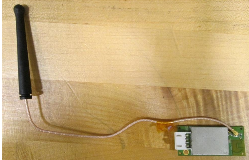
Board #8 (2.4GHz board), Shown with antenna connected.
