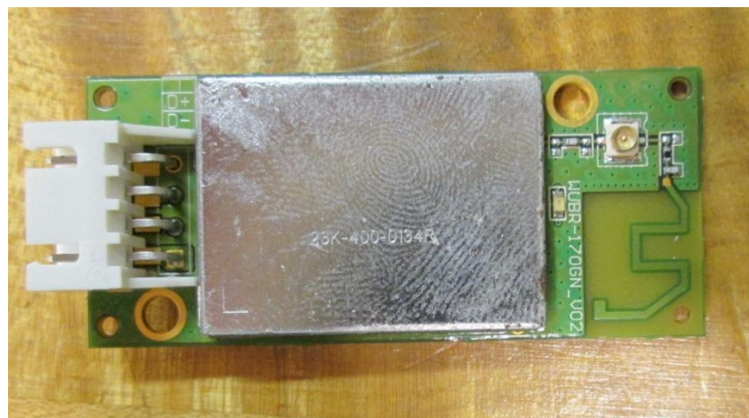
Board #8 (2.4GHz board) as seen in previous photo. Side 1.
