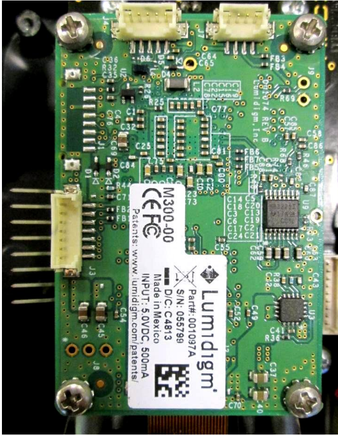
Board #1 (fingerprint reader board) as seen in photos EUT – Internal view 1-4 Side 1
