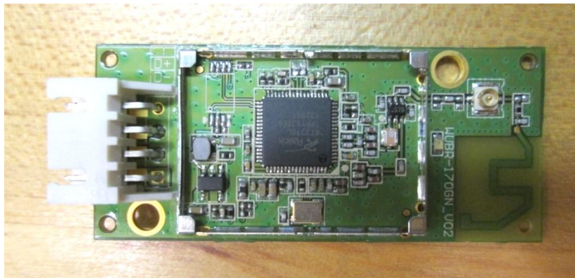
Board #8 (2.4GHz board), Side 1, Shield removed
