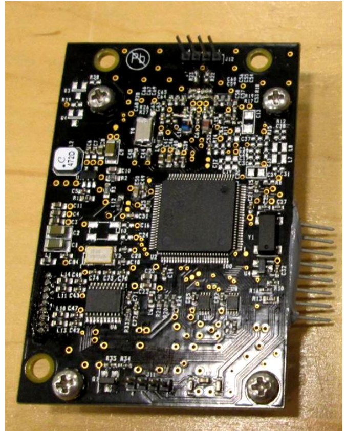
Board #2 (RFID card reader) as seen in photos EUT – Internal view 2-4 Side 2
