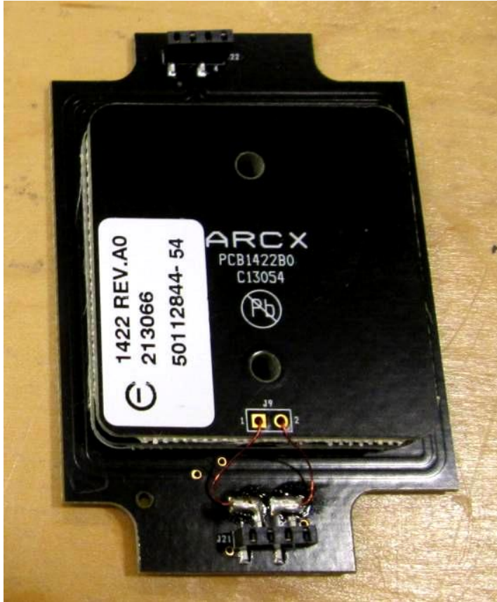
Board #3 (RFID card reader antenna) as seen in photos EUT – Internal view 3-4 Side 1
