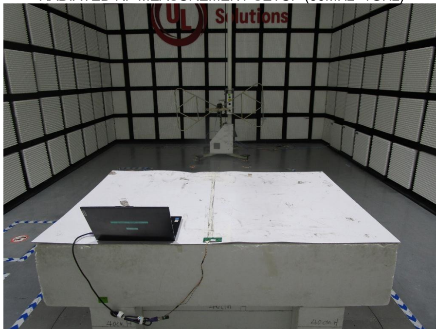
RADIATED RF MEASUREMENT SETUP (Below 30MHz)
