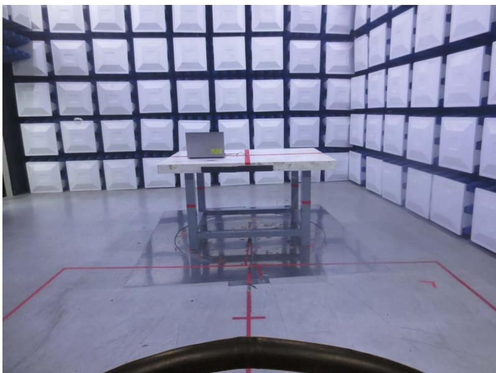
**Radiated Emissions Test Photos****30 MHz to 1 GHz**
