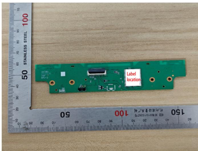
Permanent adhesive type is used to fix the label ,the label drawing isn't removed easily.
