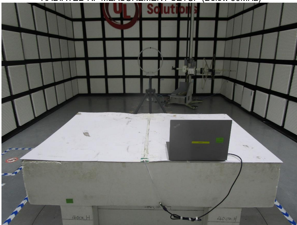
RADIATED RF MEASUREMENT SETUP (Below 30MHz)
