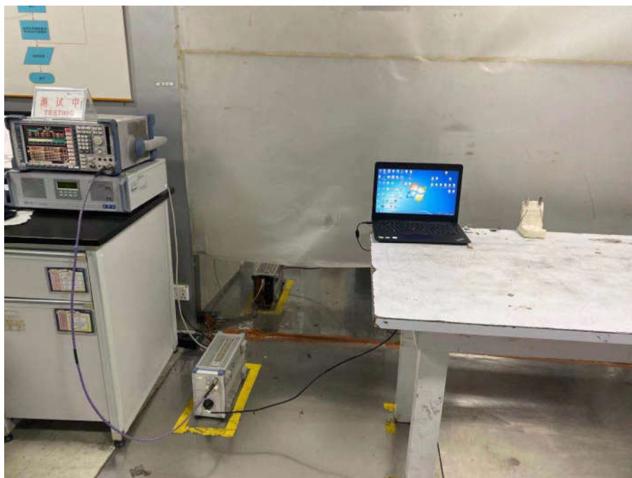
Conducted Emissions Test Setup-7
