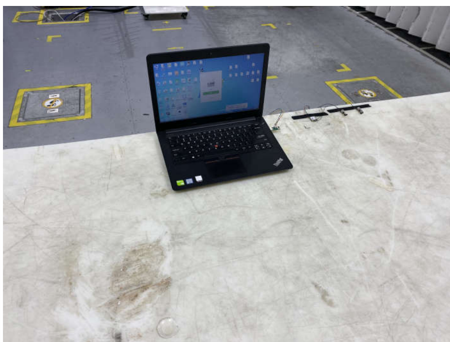
Radiated spurious emission Test Setup-3/4(Below 1GHz)
