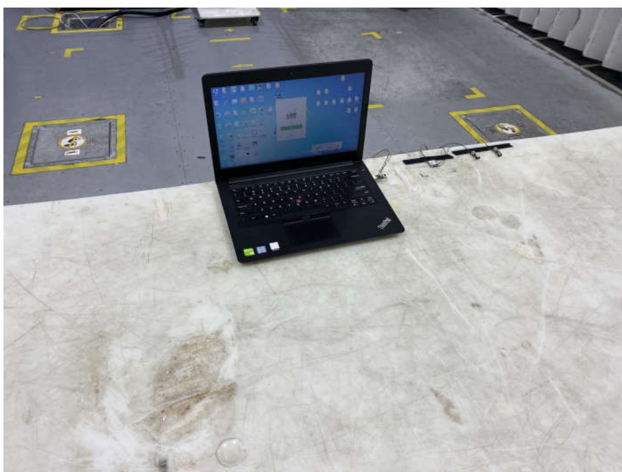
Radiated spurious emission Test Setup-1/2(Below 30MHz)
