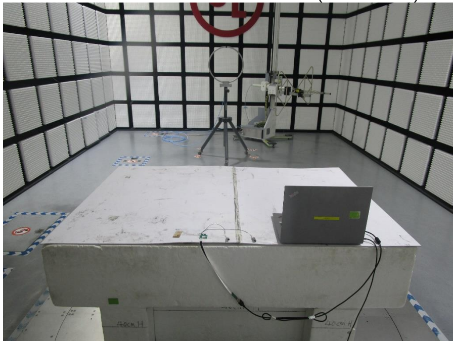
RADIATED RF MEASUREMENT SETUP (Below 30MHz)
