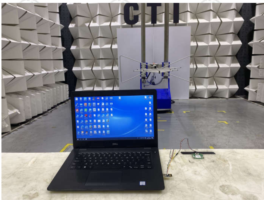
Radiated spurious emission Test Setup-2(Below 1GHz)
