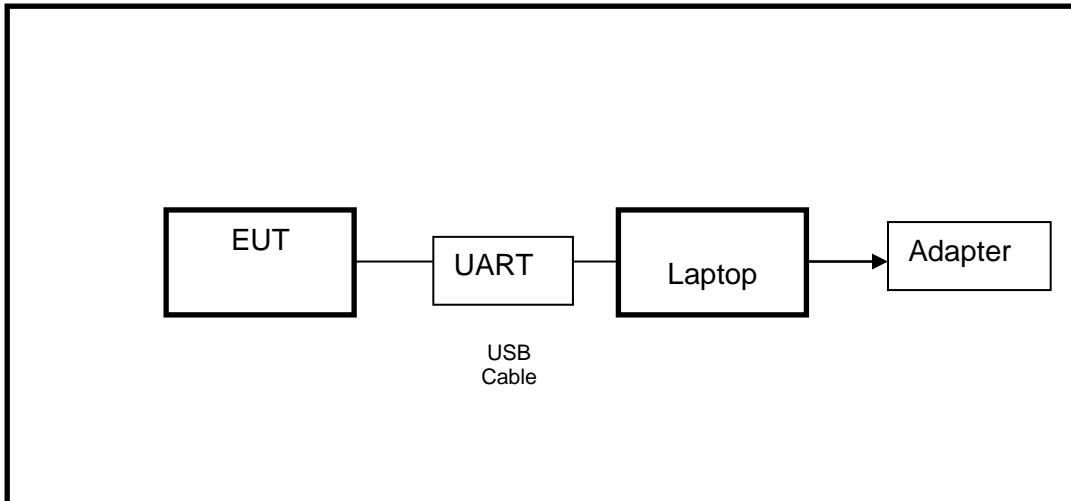
Note: AC adapter only use for AC POWER LINE CONDUCTED EMISSIONS testing.
