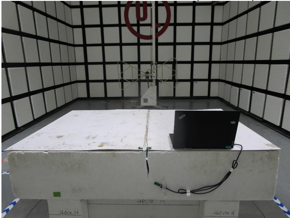
RADIATED RF MEASUREMENT SETUP (30MHz~1GHz)
