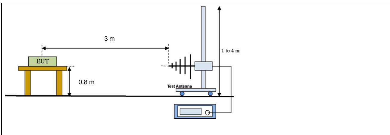
Radiated emission setup, Above 1 GHz
