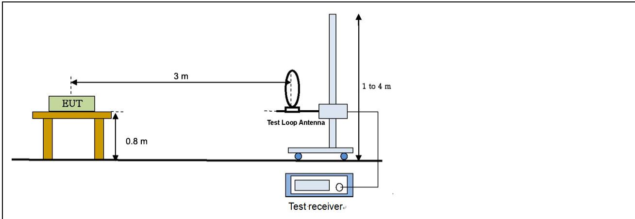
Radiated emission setup, Below 1 000 MHz
