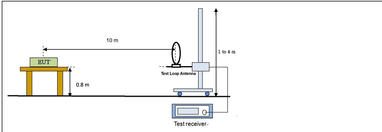
Radiated emission setup, Below 1 000 MHz
