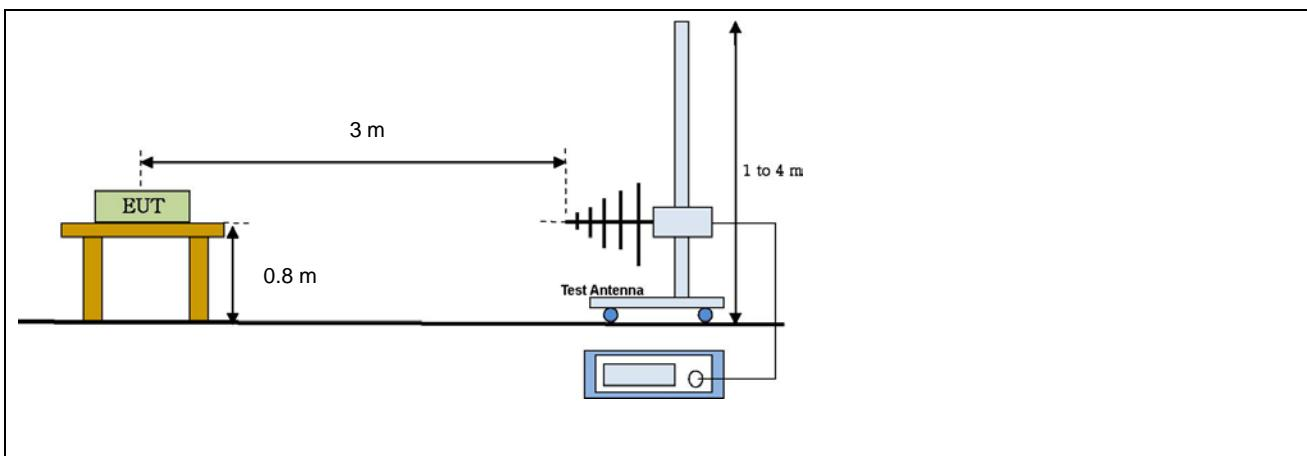
Radiated emission setup, Above 1 GHz
