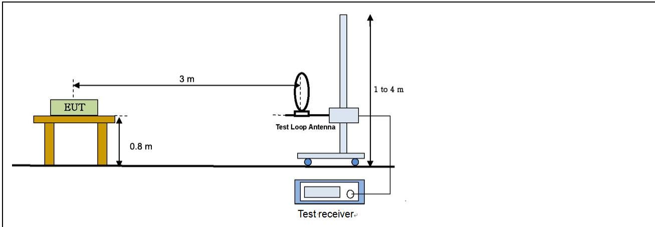
Radiated emission setup, Below 1 000 MHz
