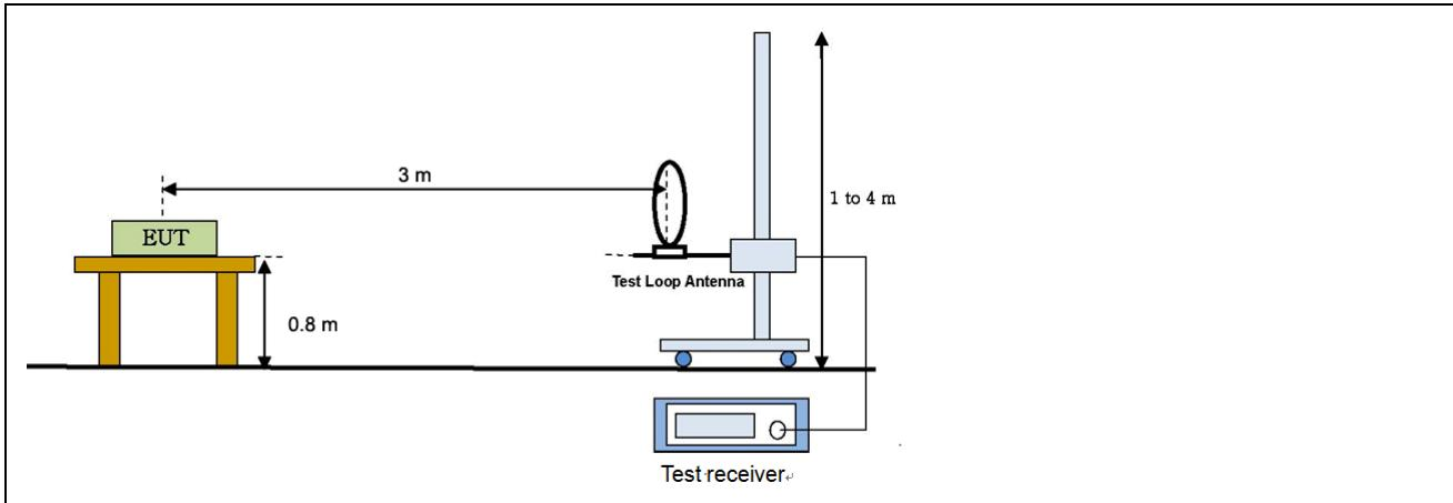
Radiated emission setup, Below 1 000 MHz
