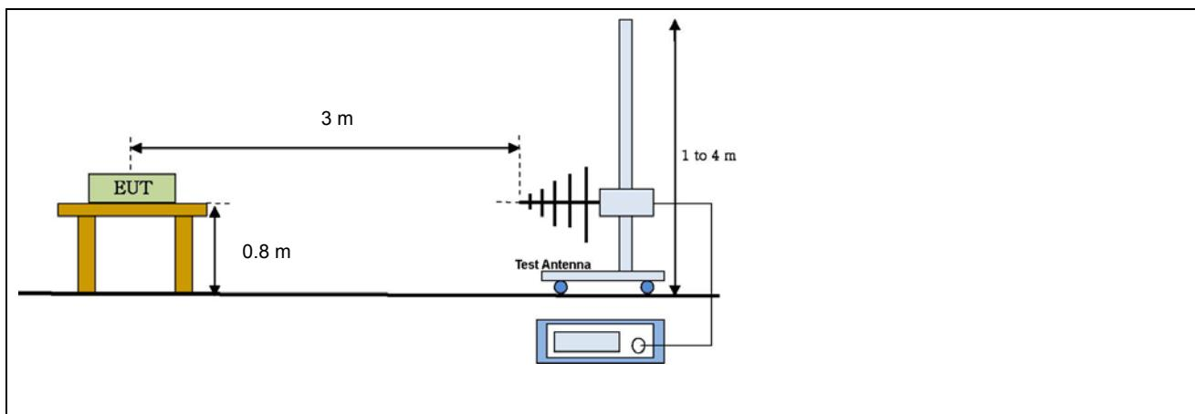
Radiated emission setup, Above 1 GHz
