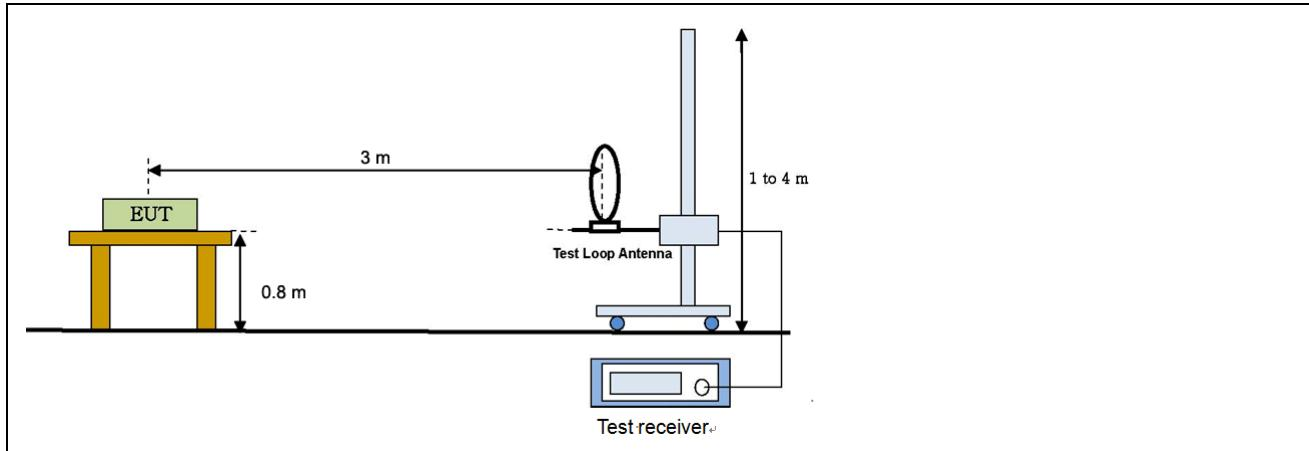
Radiated emission setup, Below 1 000 MHz
