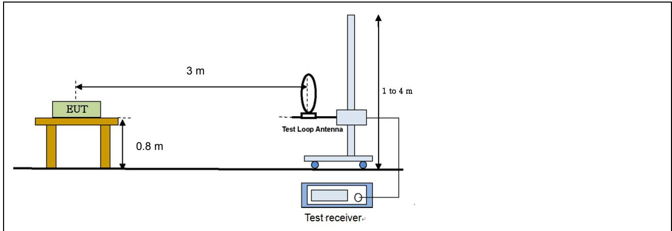
Radiated emission setup, Below 1 000 MHz
