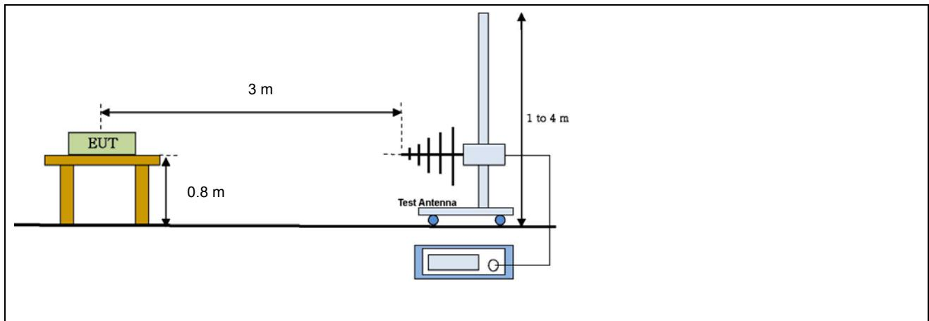
Radiated emission setup, Above 1 GHz
