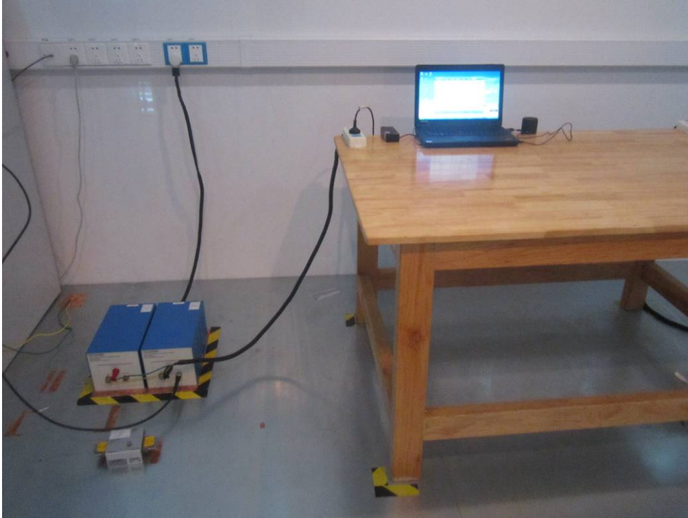
Conducted Emissions Test Setup Front View
