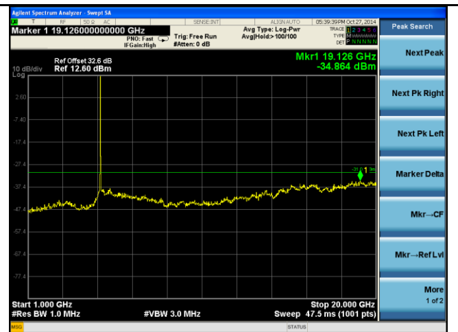
Chain 4 CSE - Mid CH 4965MHz (1GHz-20GHz)
