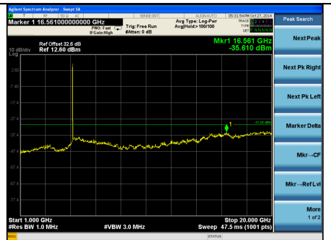
Chain 2 CSE - Mid CH 4965MHz (1GHz-20GHz)
