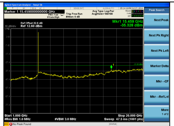
Chain 3 CSE - High CH 4980MHz (1GHz-20GHz)
