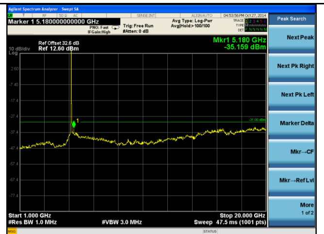
Chain 1 CSE - High CH 4980MHz (1GHz-20GHz)
