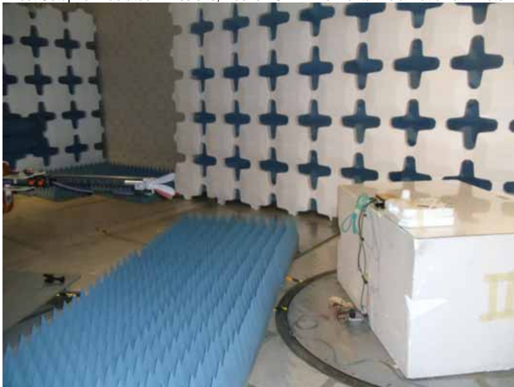
Test Setup for Radiated Emissions, Above 1GHz – Vertical Polarization at 1Meter
