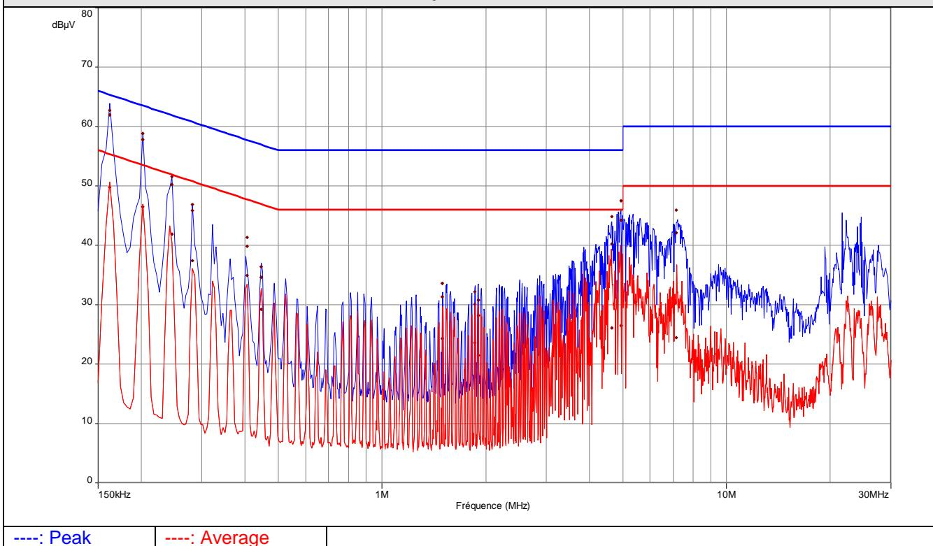
Graphical representation of Conducted Disturbance Measurement (Peak and Average detection)
