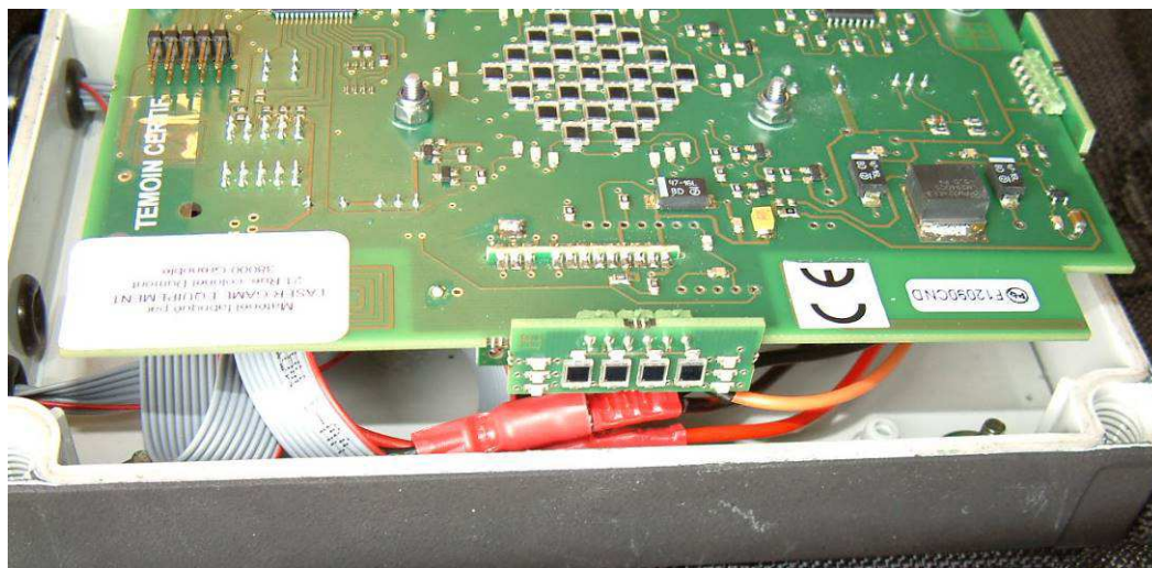
Laser detectors on PCB edges
