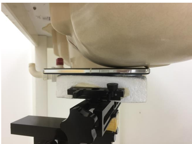
Left Cheek, Test Separation 0 mm
