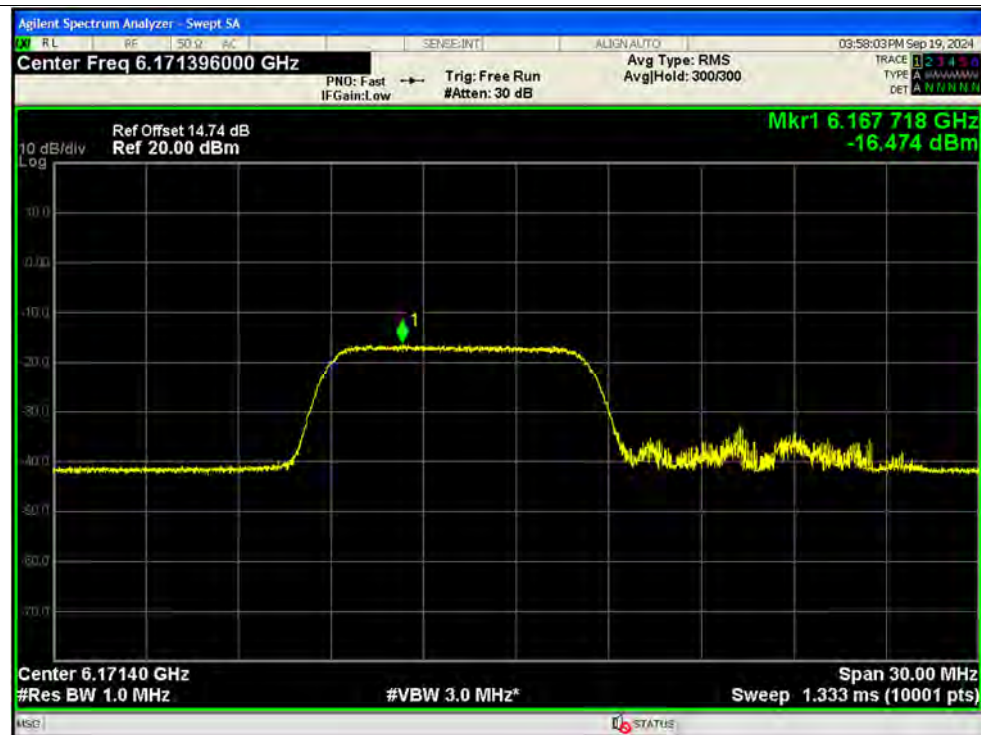
PSD NVNT ax20 106@53 6175MHz Ant13 MIMO
