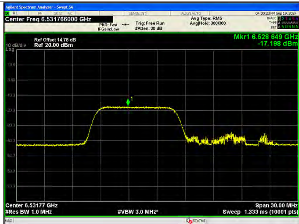
PSD NVNT ax20 106@53 6535MHz Ant13 MIMO
