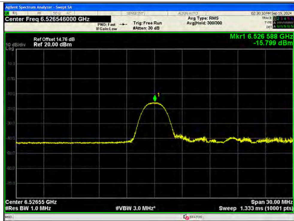
PSD NVNT ax20 26@0 6535MHz Ant13 MIMO
