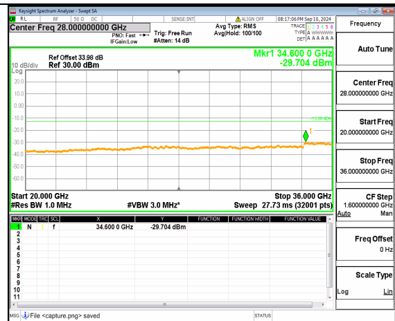
n77(3450-3550MHz) (20GHz-36GHz) 90M DFT-s-OFDM BPSK Inner_1RB_Right Low
