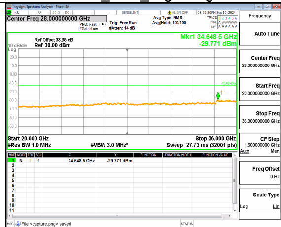
n77(3450-3550MHz) (20GHz-36GHz) 90M DFT-s-OFDM QPSK Inner_1RB_Left High
