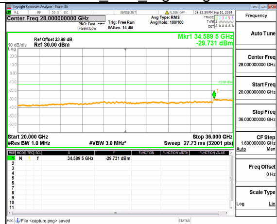
n77(3450-3550MHz) (20GHz-36GHz) 100M DFT-s-OFDM BPSK Inner_1RB_Left_Mid
