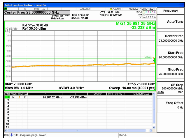
2A-7A-20G-26G / 20+20MHz / QPSK / Low+High CH / 1@0-1@99
