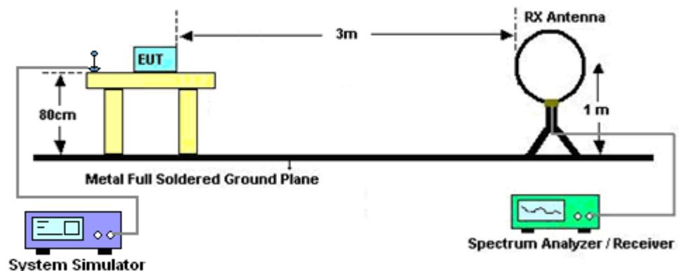
For radiated test from 30MHz to 1GHz
