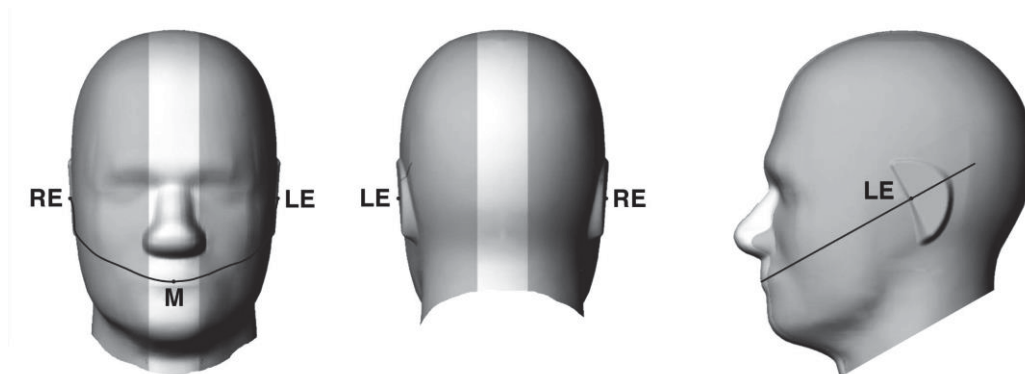
Fig 9.1.1 Front, back, and side views of SAM twin phantom
