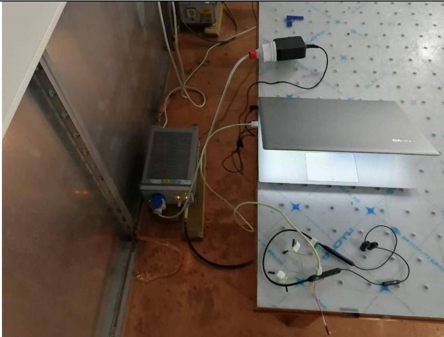
Conducted Emissions Test Setup (with charger)
