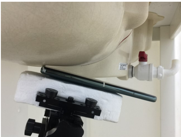
Right Tilted, Test Separation 0 mm
