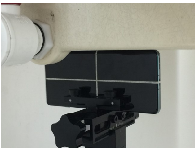
Right Side, Test Separation 0 mm
