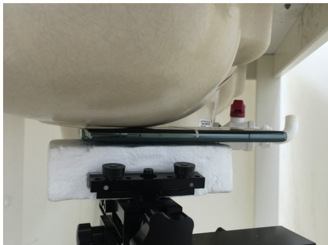
Right Cheek, Test Separation 0 mm
