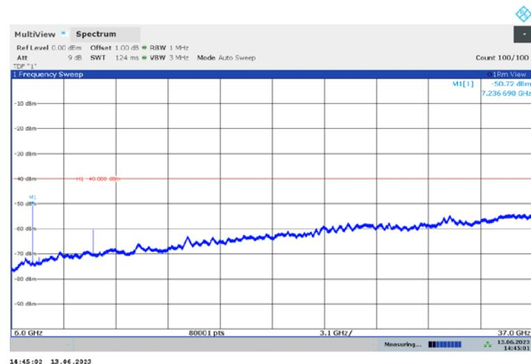
**LTE CA band 66C****NOTE: peak above the limit line is the carrier frequency.**
