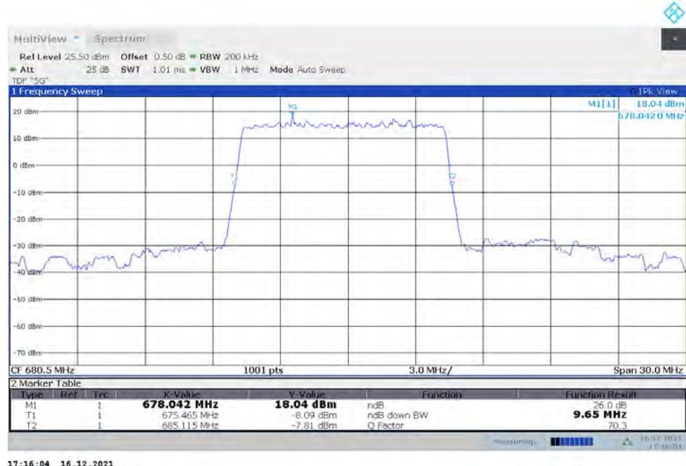
**n71,10MHz Bandwidth,DFT-s-QPSK (-26dBc BW)**
