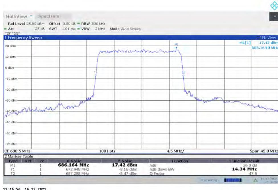
**n71,15MHz Bandwidth,DFT-s-QPSK (-26dBc BW)**
