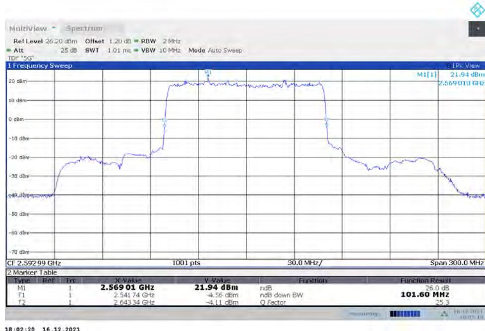
**n41,100MHz Bandwidth,DFT-s-QPSK (-26dBc BW)**
