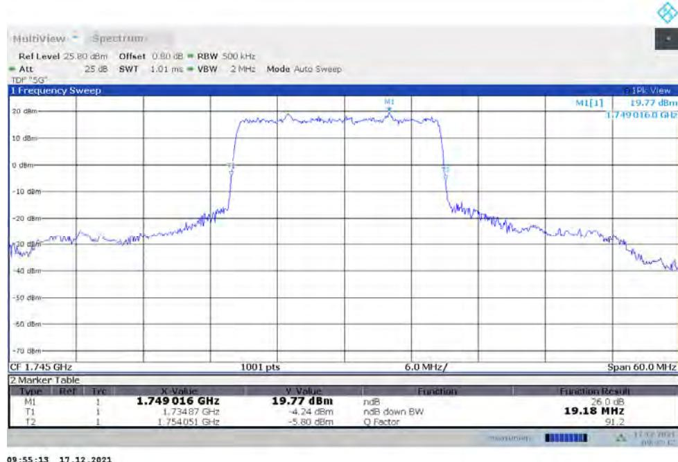
**n66,20MHz Bandwidth,DFT-s-QPSK (-26dBc BW)**
