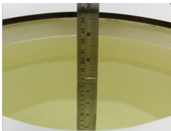
Fig 12.2 Photo of Liquid Height for Body SAR
