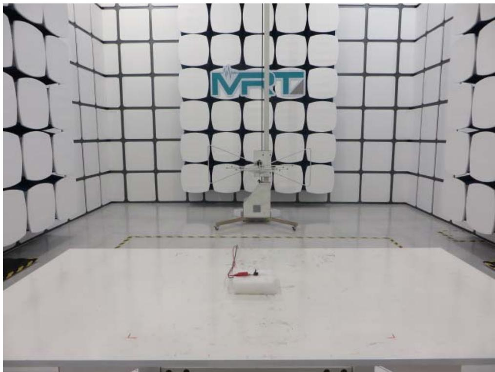
2. Description: Radiated Emission Test Setup for 1GHz ~ 18GHz
