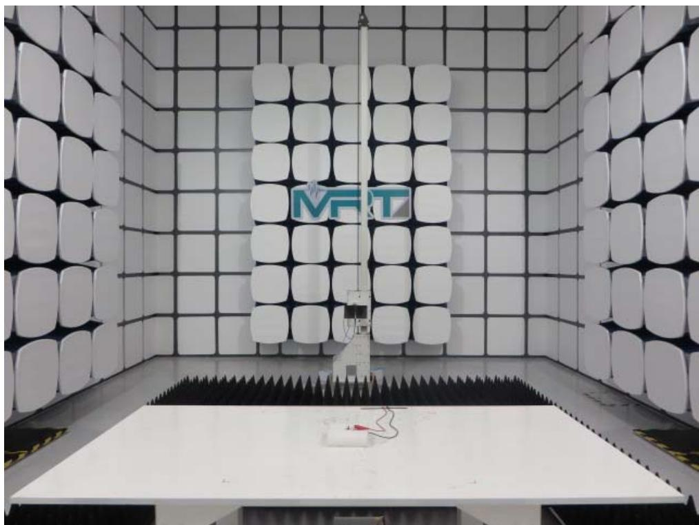
3. Description: Radiated Emission Test Setup for 18GHz ~ 40GHz
