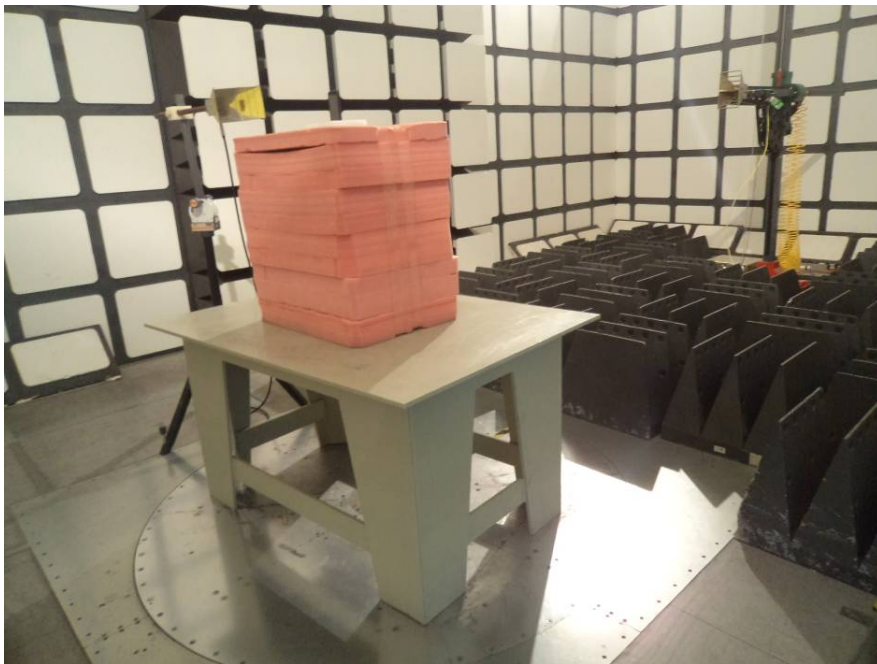
Radiated Emissions Test View (Above 1 GHz)
