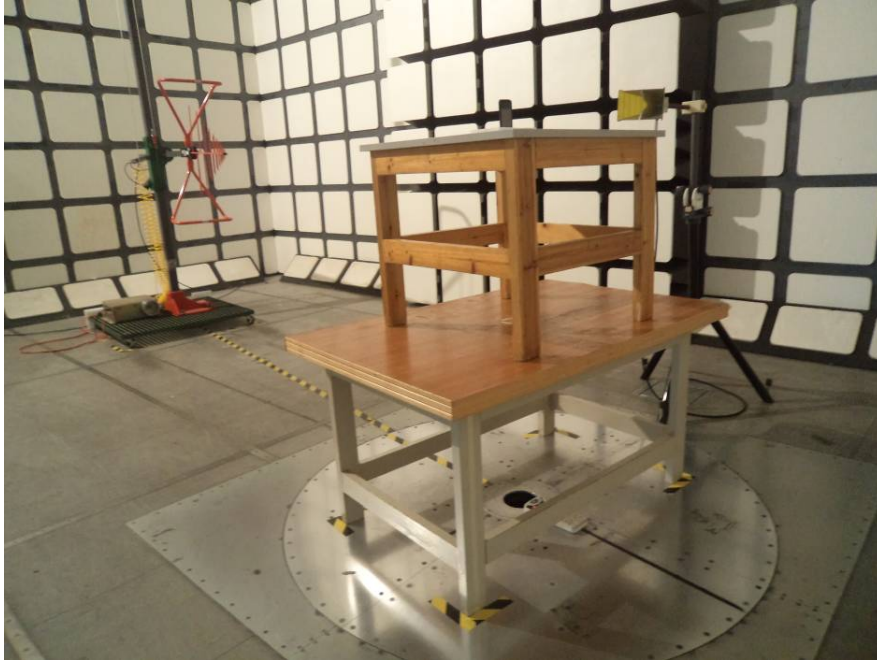
Radiated Emissions Test View (Below 1 GHz)
