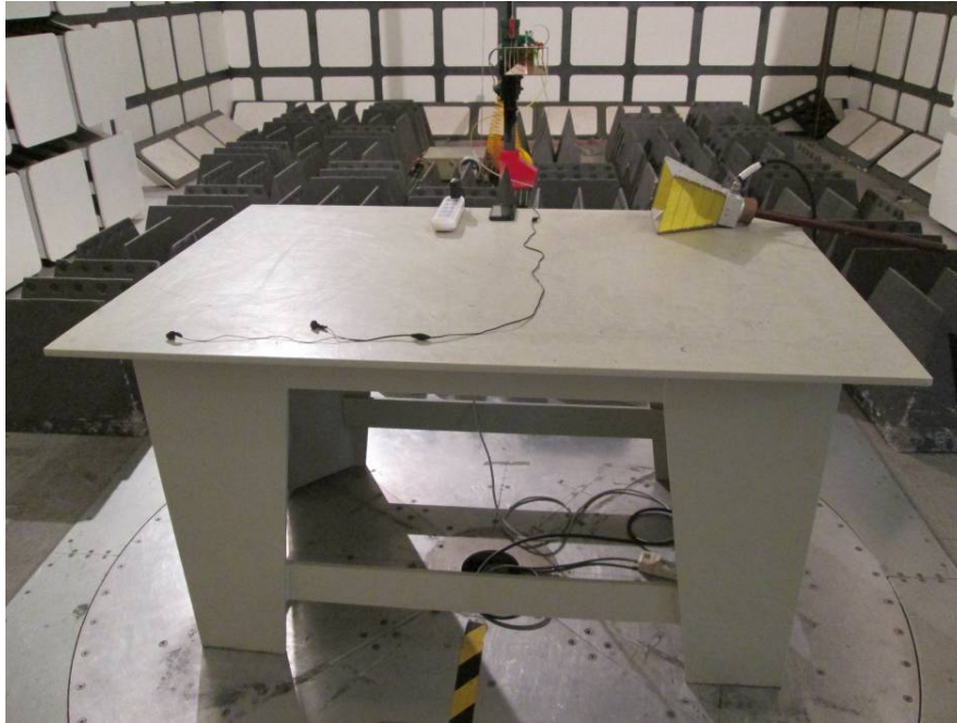
Radiated Emissions – Front View (1-25 GHz)
