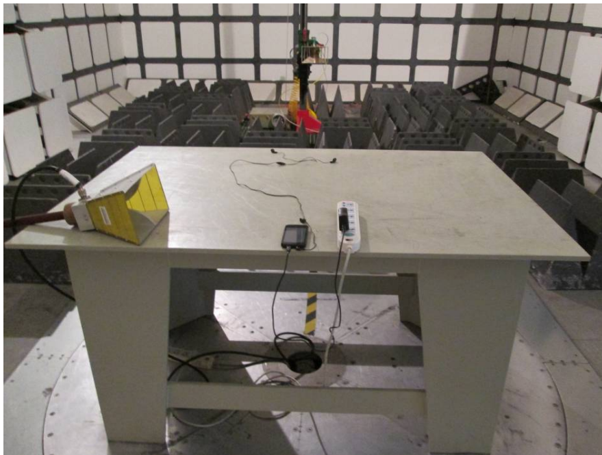
Radiated Emissions – Rear View (1-25 GHz)
