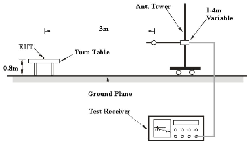
The radiated emission tests were performed in the 3-meter chamber a test site, using the setup accordance with the ANSI C63.10. The specification used was the FCC Part Subpart C limits.
