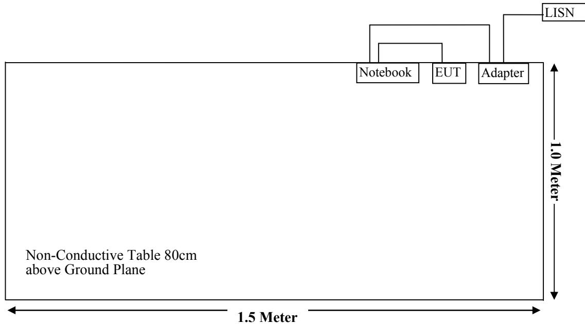
For Radiated Emissions (Below & Above 30MHz):
