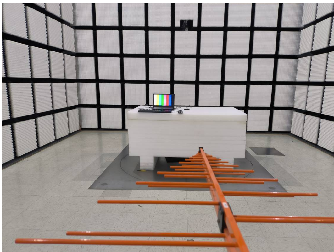
Radiated Emission Below 1GHz View Parallel
