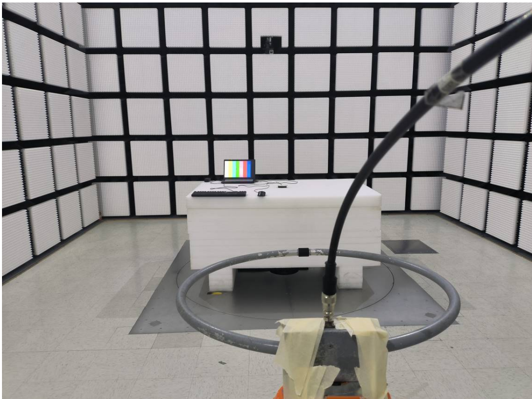
Radiated Emission Below 1GHz View Ground-parallel
