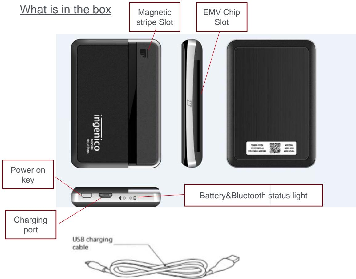
This card reader supports the acceptance of EMV® chip cards, magnetic stripe cards. It is certified and compliant with industry payment standards: EMV Level 1 / EMV Level 2 / TQM, FCC / RoHS / WEEE.
