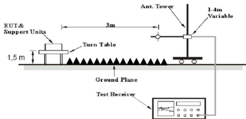
The radiated emission tests were performed in the 3 meters chamber test site, using the setup accordance with the ANSI C63.10-2013. The specification used was the FCC 15.209, and FCC 15.247 limits. The external I/O cables were draped along the test table and formed a bundle 30 to 40 cm long in the middle.
