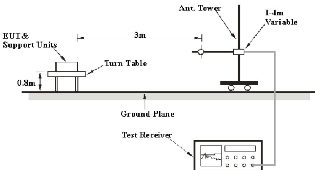
The radiated emission tests were performed in the 3 meters chamber test site, using the setup accordance with the ANSI C63.4-2014. The specification used was the FCC Part 15.109 limits.
