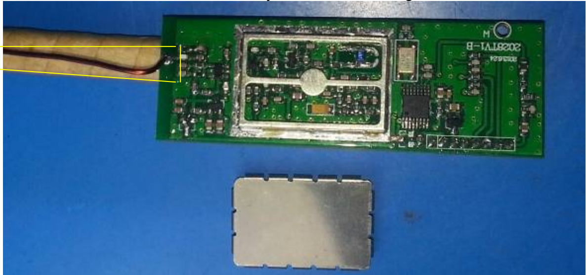
U-6298 with PCB Layout's Antenna: Length: 5cm
