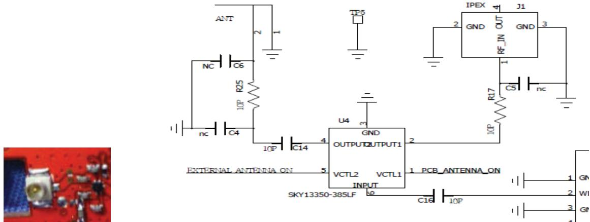
The above diagram shows the connector (J1) is by default disabled by the SKY13350-385LF (U4) switch, therefore, the circuitry is open. During normal operations, there is no signal OUTPUT through the connector (J1) permanently for end product.
