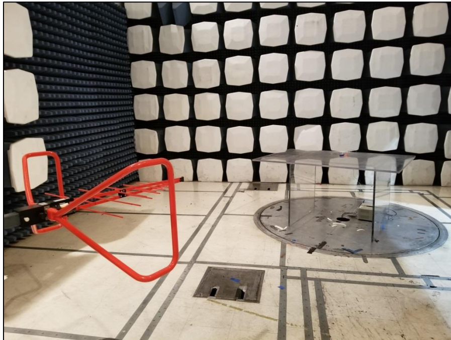
Photograph 2. Radiated Spurious Emissions, Below 1 GHz, Test Setup
