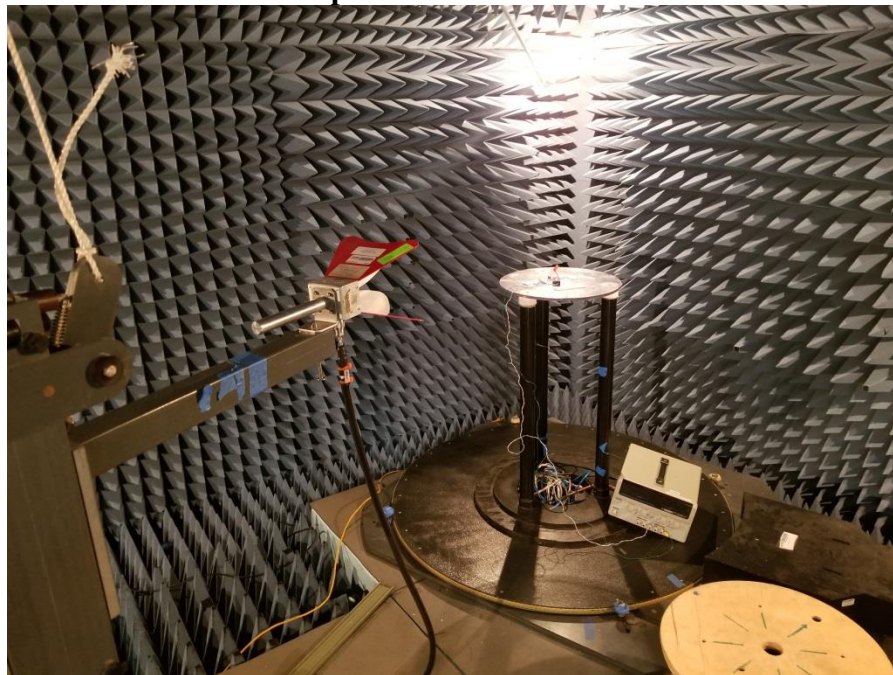
Photograph 1. Radiated Spurious Emissions, Above 1 GHz, Test Setup
