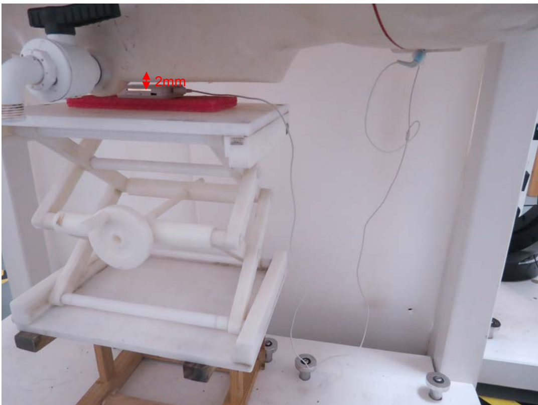
Picture 18: Back Side with earphone without strap attached, the distance from handset to the bottom of the Phantom is 2mm
