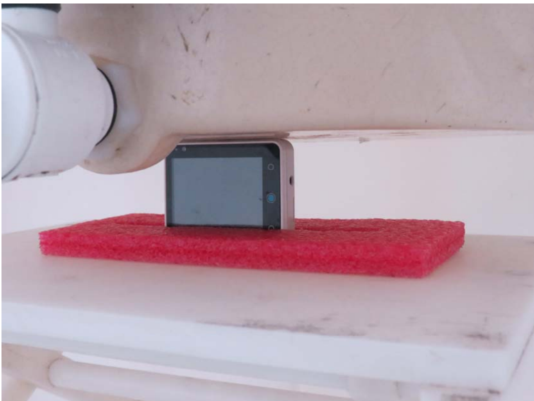
Picture 16: Top Edge without strap attached, the distance from handset to the bottom of the Phantom is 0mm
