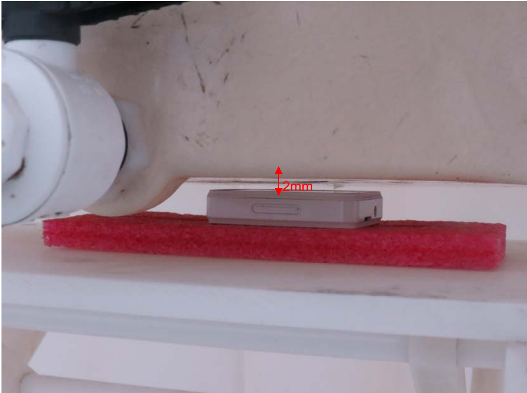
Picture 13: Front Side without strap attached, the distance from handset to the bottom of the Phantom is 2mm
