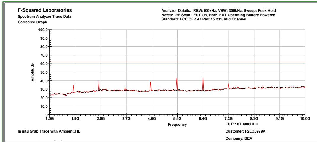
**Characterization Scan, Mid Channel: 1 GHz to 10 GHz, Vertical**
