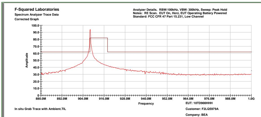
**Characterization Scan, Low Channel: 900 MHz to 1 GHz, Vertical**
