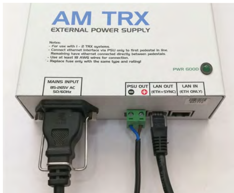
Picture 1 - Connected external power supply
