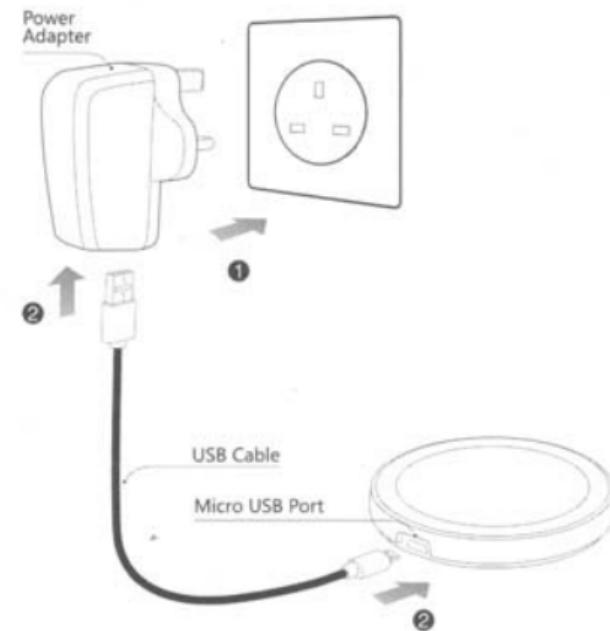
① Connect the power adapter to socket.
