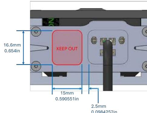
**Connections:** Insert power cable, 2x2 Molex Power Connector and Mounting Panel, onto the back plane of the reference chassis ensuring the alignment of the plate, connector and cover, and tighten the four (4) #2-56  $\frac{3}{8}$ " screws to a torque of 3 in-lbs. The push-in connector is now installed.
