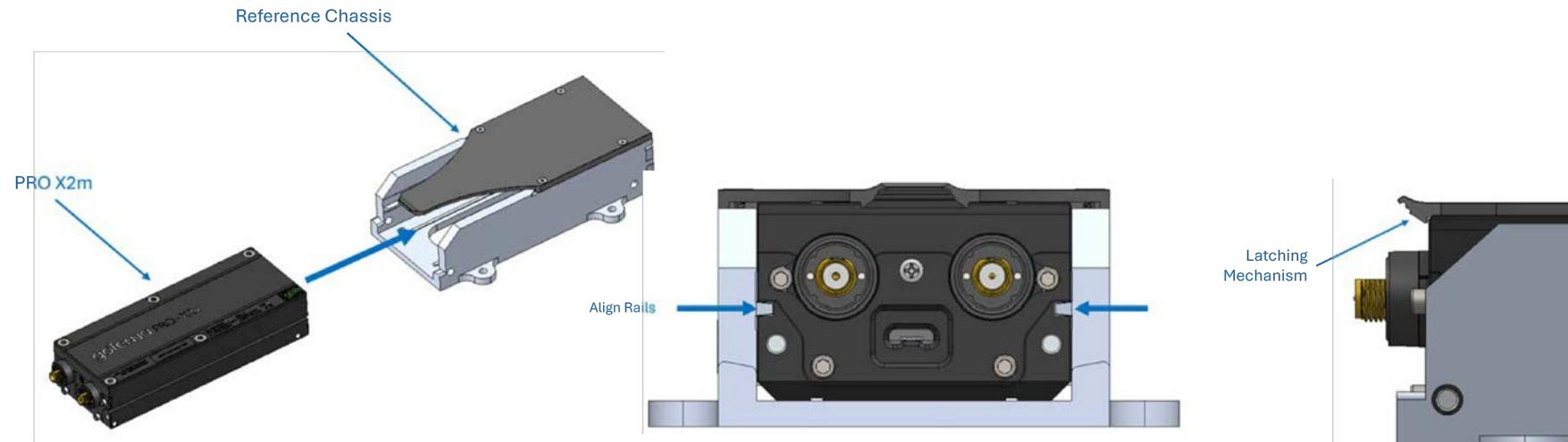
**Ensure alignment:** Ensure The frontplane with RF out is exposed to the user while the backplane with power is aligned with the chassis power interface. Utilize a locking or latching mechanism to ensure the Pro-X2m remains properly seated.
