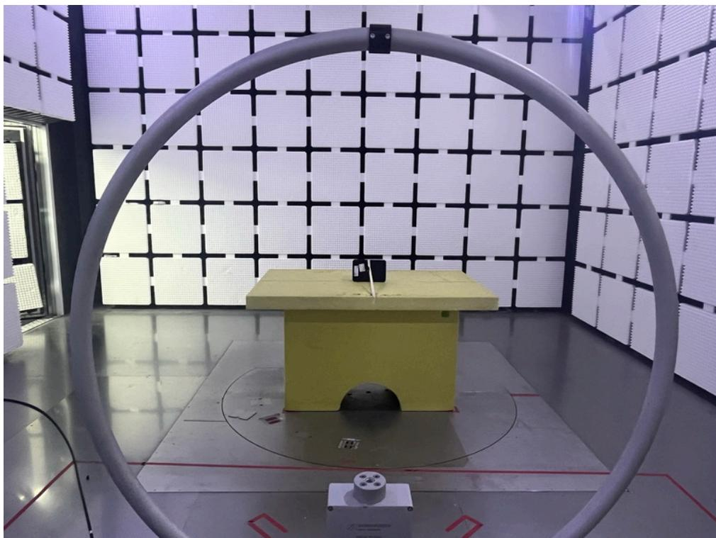
**Radiated Emissions Test Photos****30 MHz to 1000 MHz**
