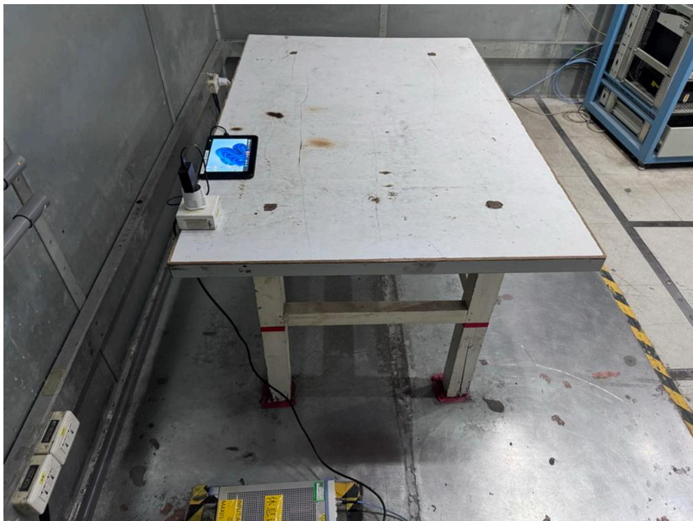
**Radiated Emissions Test Photos****9 kHz to 30 MHz**
